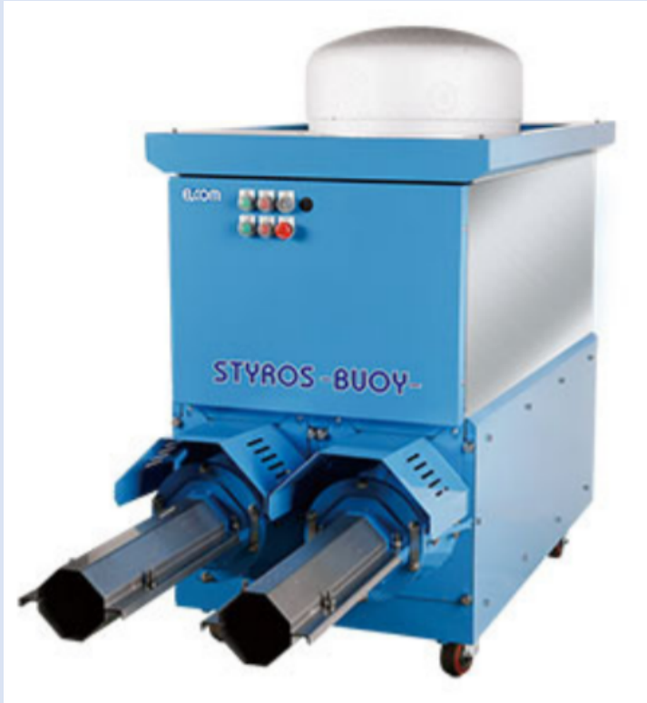
Machine for compressing EPS used in demonstration project.
