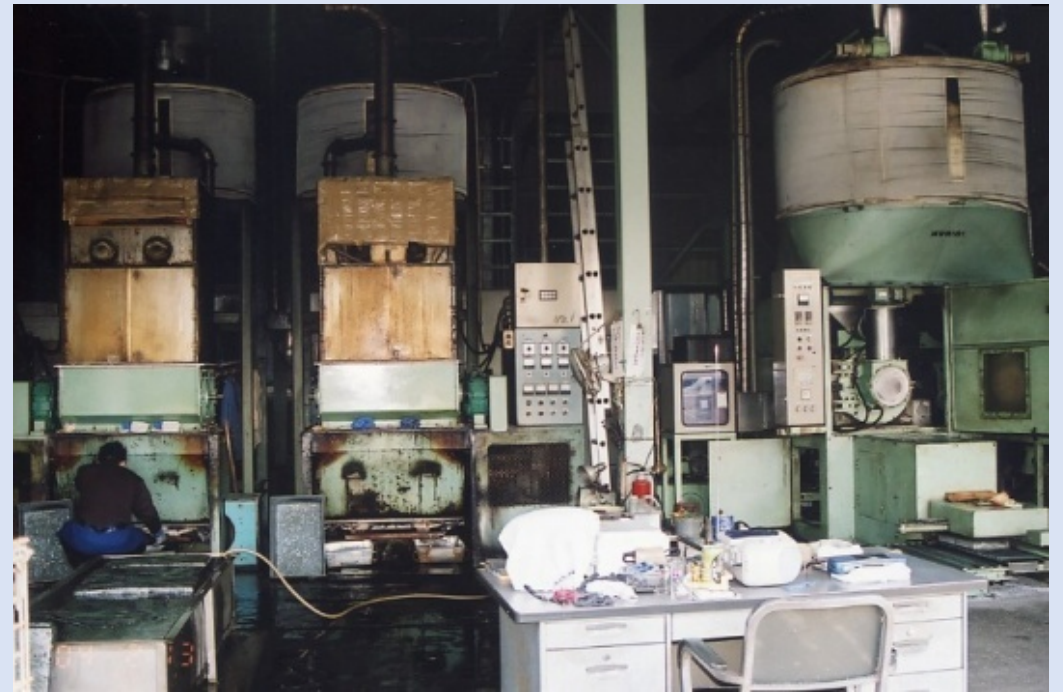
↑ Machines compressing EPS Fish Boxes at Tsukiji Fish Market in 2004.
